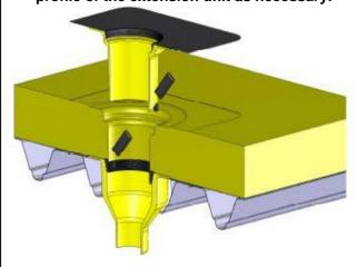
6). Shorten the extension unit if necessary and apply the enclosed lubricant to the rubber sealing ring and the bottom of the extension unit. The extension unit should go past the bottom of the rubber sealing ring to ensure a good fit.
