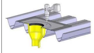
4). Install the vapour control layer and seal to the outlet flange using butyl tape if using Spectravap VCL or by hot air welding / torch-on application if an IKO bituminous VCL is being used.
