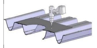
3). Install the IKO Trendy outlet and mechanically fasten to the substrate with appropriate IKOfix fasteners.
