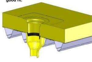
7). Install the extension unit by pushing through in to the rubber sealing ring and secure by fixing the membrane flange to the substrate using IKOfix fasteners and IKOfix GOK thermally broken pressure plates.
