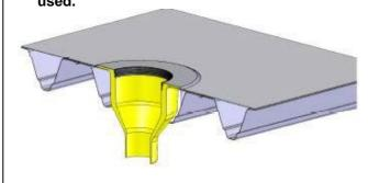
5). Install the rubber sealing ring into the outlet opening.
