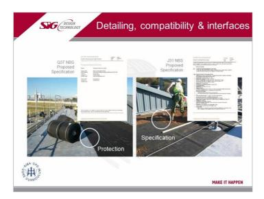
These two images show where the integrity of the membrane can compromise the NBS specification by puncturing the membrane, ultimately leading to water ingress
