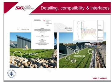
However, by using the correct materials (in the case of this membrane with a FLL certificate) and standard detailing to avoid puncturing the membrane, these roof membrane systems are not punctured at interfaces and do not risk water ingress.
