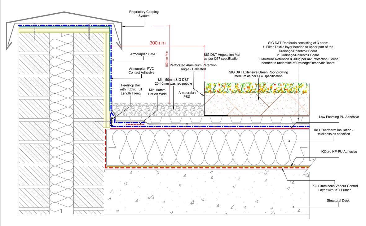
Waterproofing should be installed in accordance with BS 6229:2003 and SIG Design & Technology fixing instructions.
