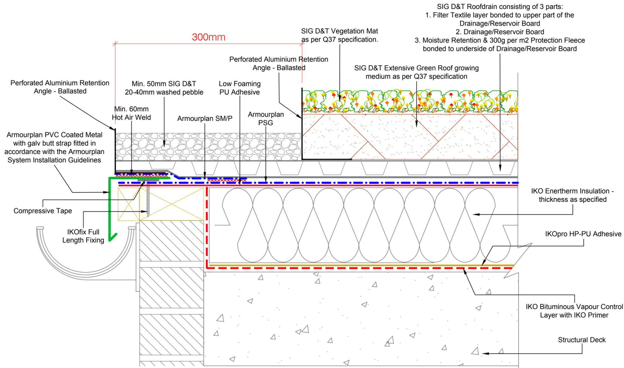
Waterproofing should be installed in accordance with BS 6229:2003 and SIG Design & Technology fixing instructions.
