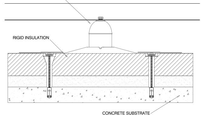
SOLAR PANEL SUPPORT POSTS FITTED IN ACCORDANCE WITH LATCHWAYS DATA SHEET NO 65616-98-4
