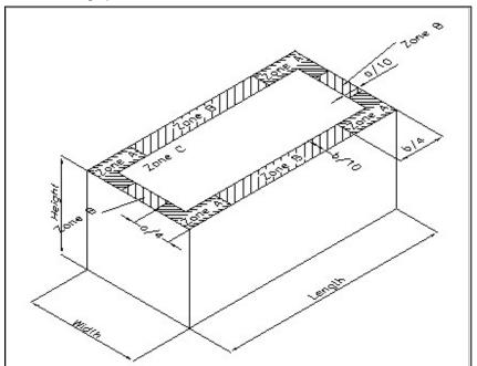
b = Length or 2 x Building Height whichever is the smaller a = Width or 2 x Building Height whichever is the smaller
