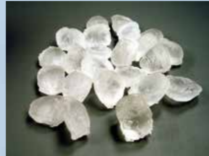
The material that makes Rhepanol roofing membranes so special: Polyisobutylene (PIB).
