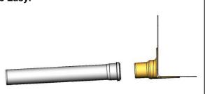
3). Secure the flange of the Easy Flow mechanically using IKOfix fasteners and pressure membrane flange. plates.
