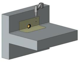
4). Hot air weld the roof membrane to the Easy Flow
