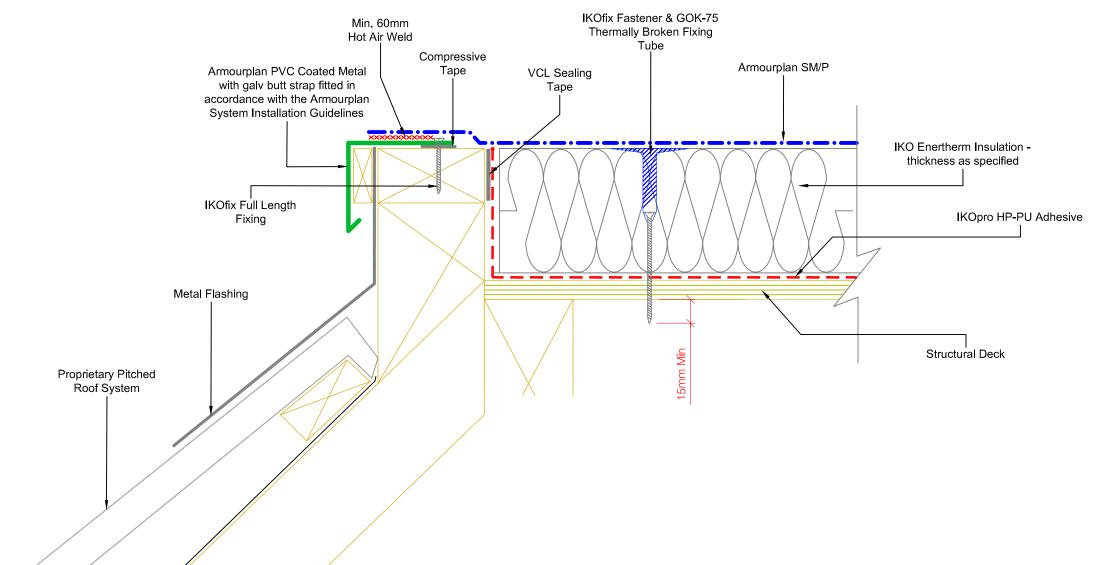
Waterproofing should be installed in accordance with BS 8000: Part 4:1989 and IKO Polymeric fixing instructions.
