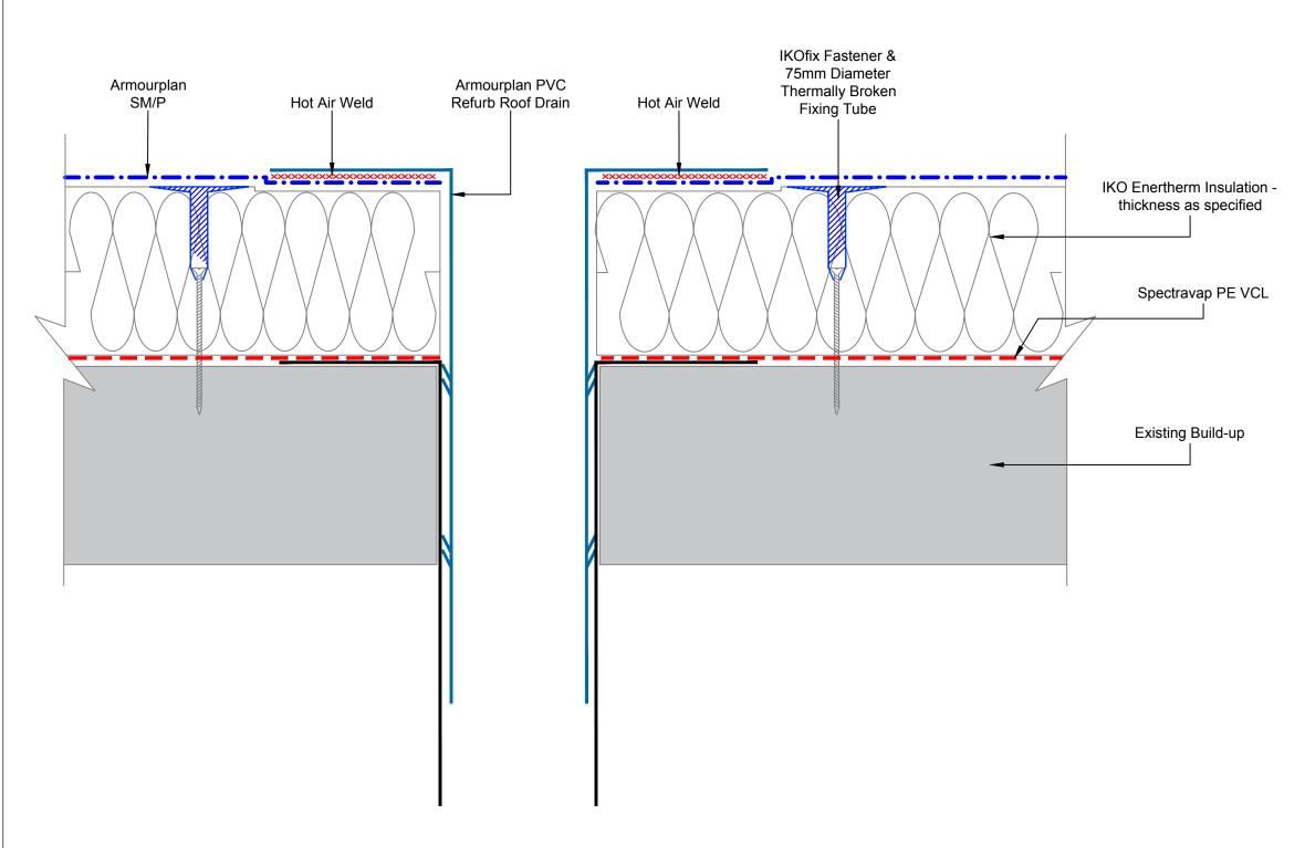
Waterproofing should be installed in accordance with BS 8000: Part 4:1989 and IKO Polymeric fixing instructions.
