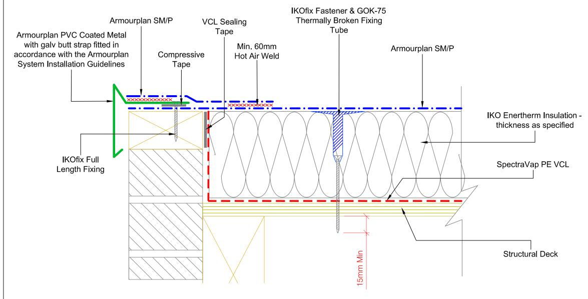
Waterproofing should be installed in accordance with BS 8000: Part 4:1989 and IKO Polymeric fixing instructions.
