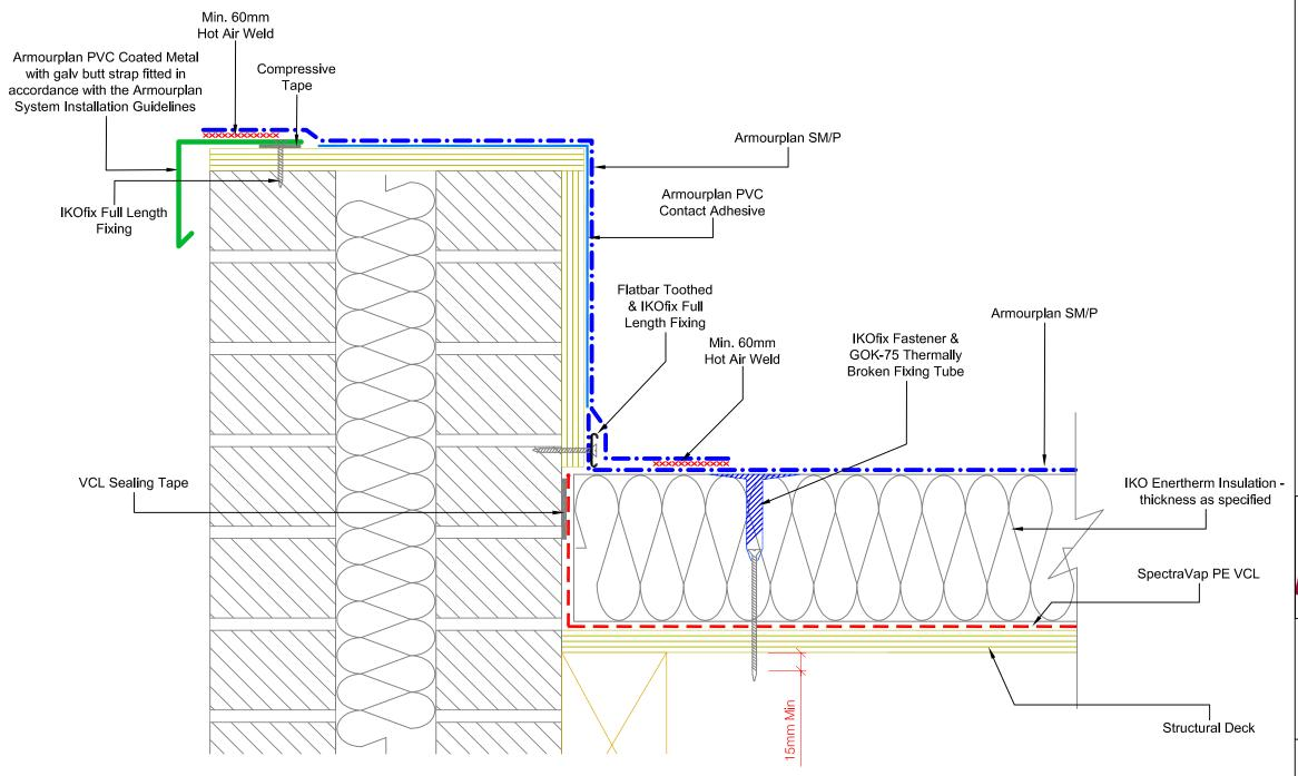
Waterproofing should be installed in accordance with BS 8000: Part 4:1989 and IKO Polymeric fixing instructions.
