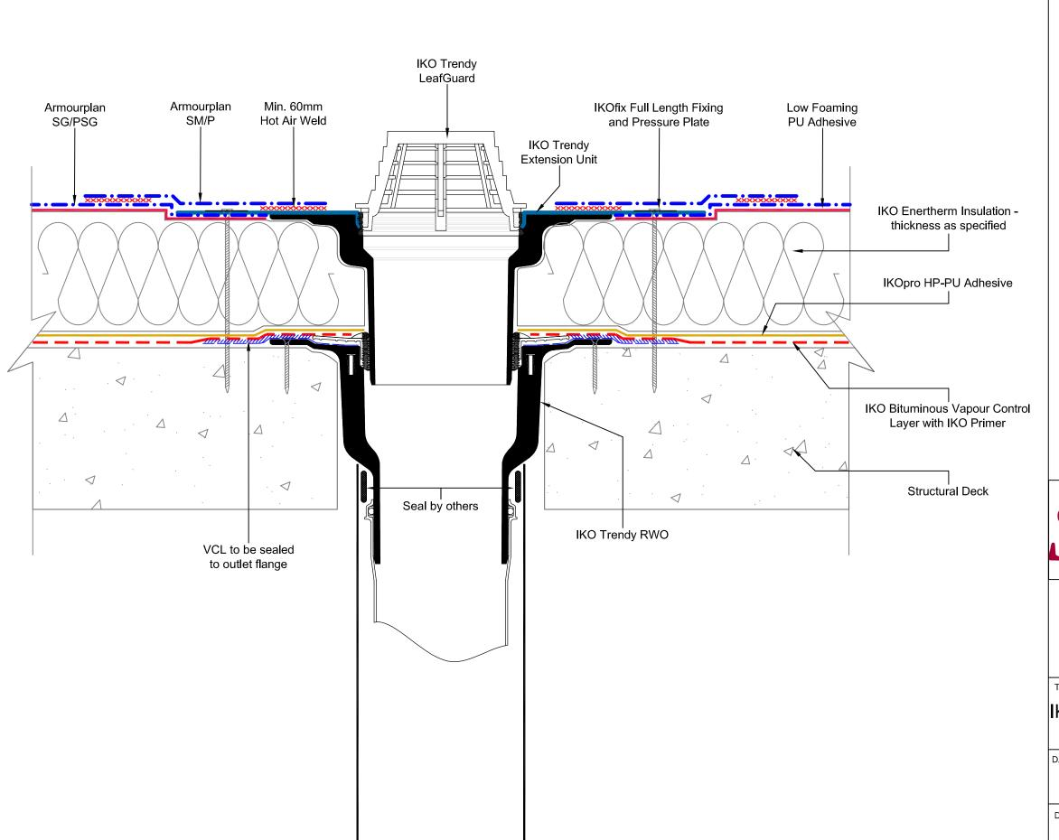
Waterproofing should be installed in accordance with BS 8000: Part 4:1989 and IKO Polymeric fixing instructions.
