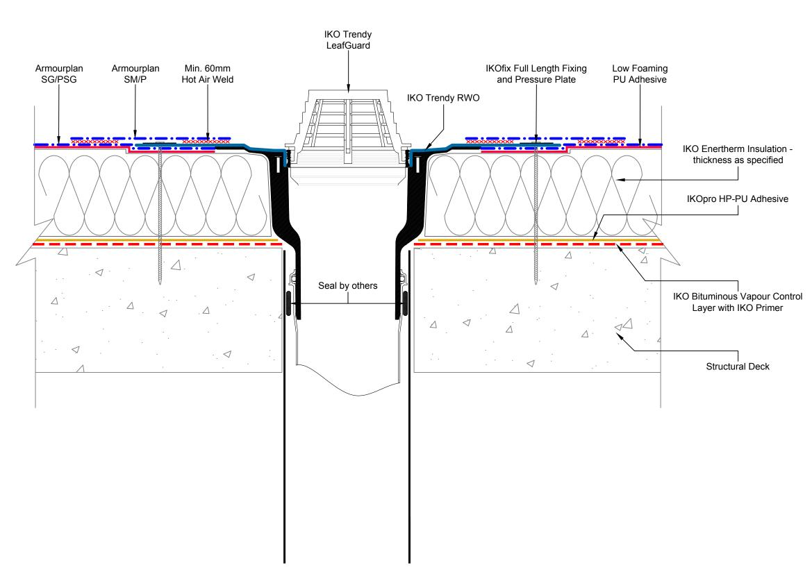
Waterproofing should be installed in accordance with BS 8000: Part 4:1989 and IKO Polymeric fixing instructions.
