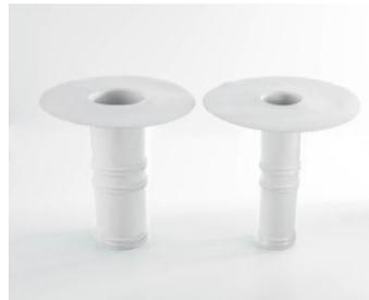
Please be advised that the Spigot (or pipe section) on Vertical Drop Armourplan Rainwater Outlets has a number of flexible rings / fins on the outside, in order ensure a tight fit inside the existing Rainwater outlet/downpipe.
