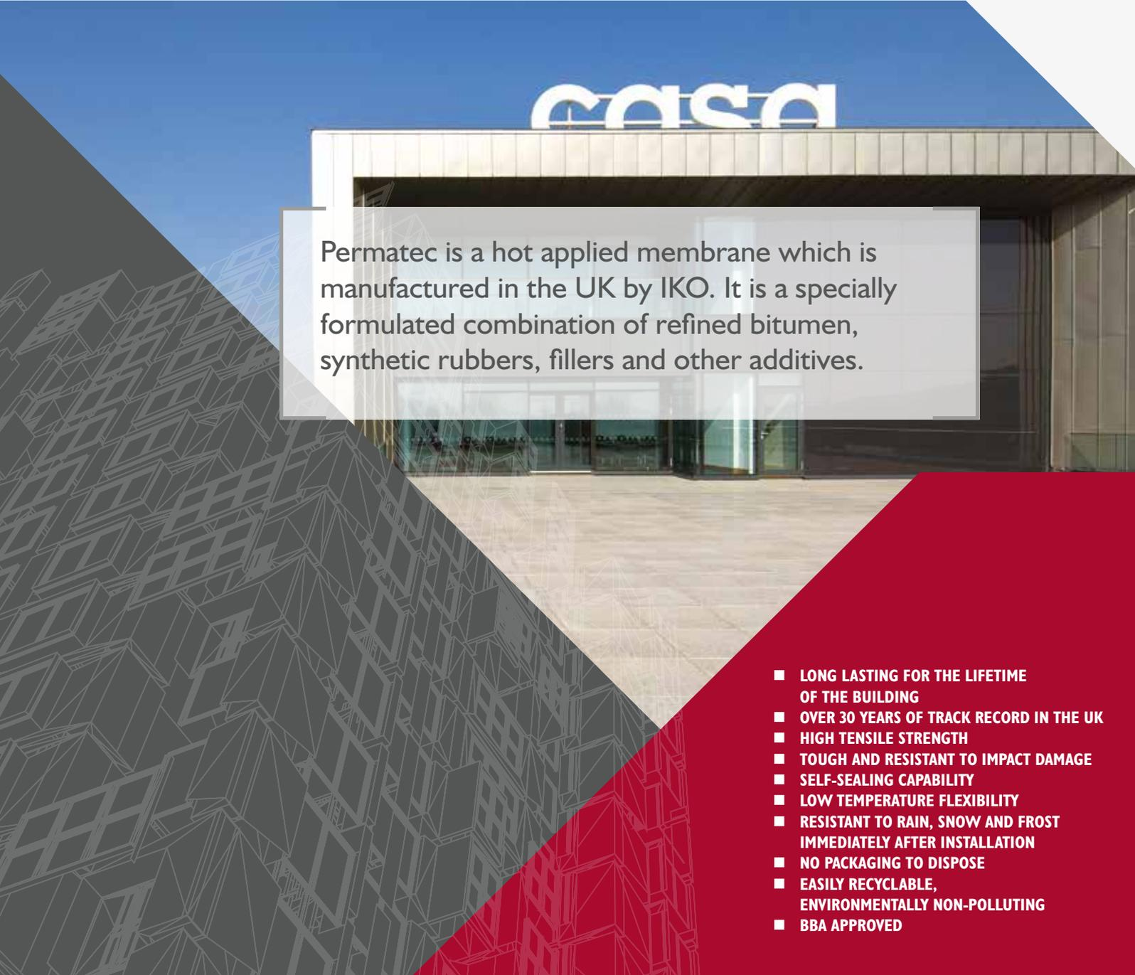
Permatec is a hot applied membrane which is manufactured in the UK by IKO. It is a specially formulated combination of refined bitumen, synthetic rubbers, fillers and other additives.
